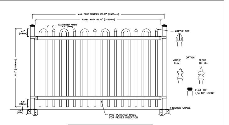
PANEL HEIGHT PANEL WIDTH POST CENTERS UP TO 6FT, HIGH 101" [2565mm] 95 ¾" [2432mm] 74 🗗 [1899mm] 7FT. AND HIGHER 80" [2032mm]
