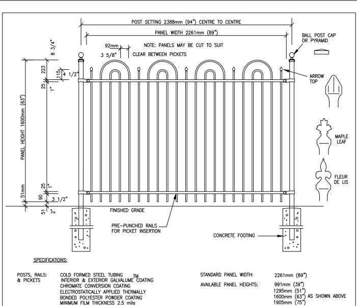
BONDED POLYESTER POWDER COATING MINIMUM FILM THICKNESS 2.5 mils
